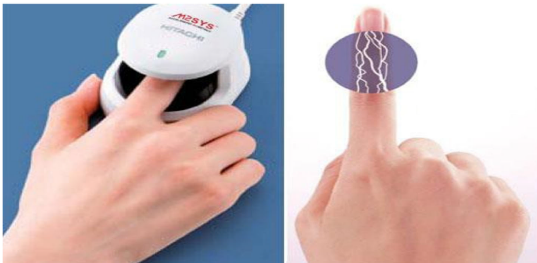
Figure 3.8: Typical finger vein readers
