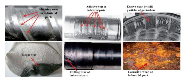
Figure 1: Some examples on the wear of industrial parts [11].
