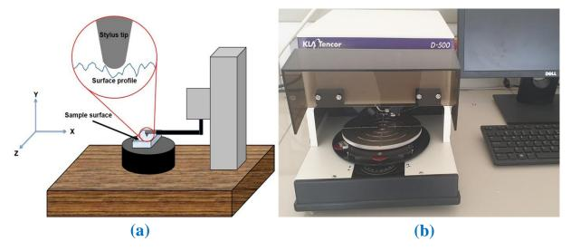
**Figure II.10:** The principle of sensor contact profilometer (a) and the used AlphaStep D-500 Stylus Profiler (b).
