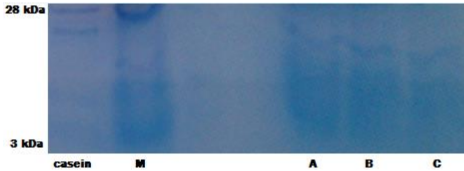
Fig.1. SDS page of camel milk casein and its pepsin hydrolysates at different hydrolysis time M : molecular weight marker, peptic hydrolysate at 60min ( A ) peptic hydrolysate at 90min ( B ), peptic hydrolysate at 120min ( C ).
