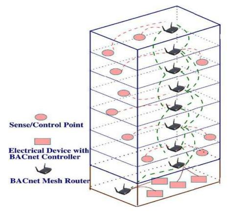
Fig. 2.10 WMNs for building automation [4]
