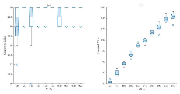
Fig. 6.9 Effect of the number of mesh clients on coverage and connectivity
