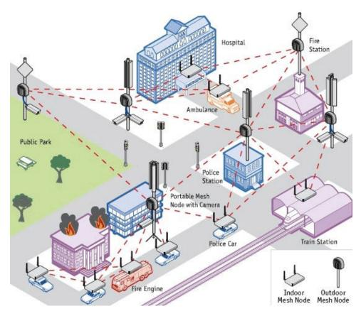
Fig. 2.2 Wireless mesh network [80]
