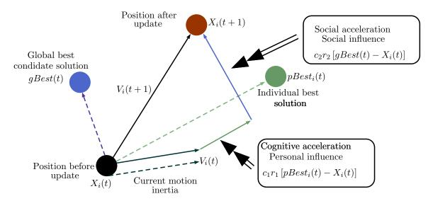
Fig. 4.11 Illustration of velocity and position updates in LDWPSO algorithm.
