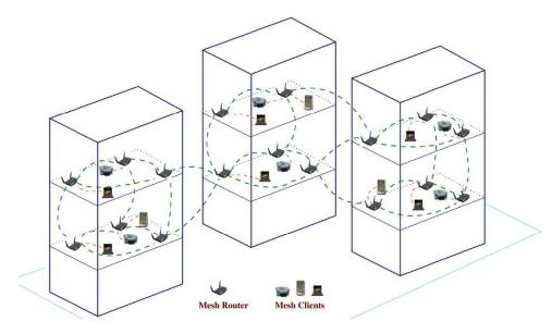
Fig. 2.7 WMNs for enterprise networking [16]
