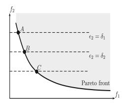
Fig. 4.7 Slicing the objective domain in the  $\varepsilon$ -constraint method.
