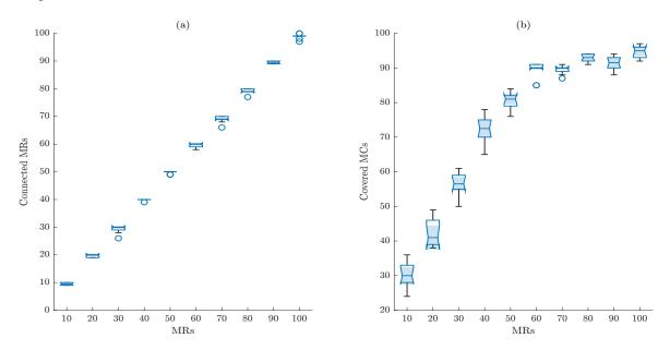
Fig. 6.8 Effect of the number of mesh routers on coverage and connectivity
