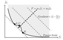
Fig. 4.4 Weighted sum method for two objectives  $f_1$  and  $f_2$  and  $w_1 + w_2 = 1$ .
