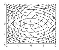
Fig. 4.3 Final locations of 40 particles after 5 iterations. The optimal point is at (1/3, 0) marked with o
