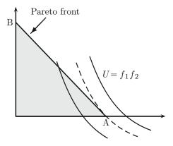
Fig. 4.6 The Pareto front is the line connecting A(5, 0) and B(0,  $5/\alpha$ ). The Pareto solution with maximum utility is  $U_* = 25$  at point A.
