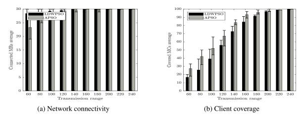
Fig. 5.10 Effect of the transmission range on coverage and connectivity
