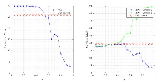
Fig. 6.4 Connected MRs/Covered MCs number vs aggregation coefficient  $\lambda$ (transmission range = 80m)
