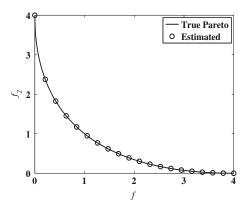
Fig. 4.9 The true Pareto front and the estimated front when setting  $f_2$  as the objective and  $f_1$  as the constraint.
