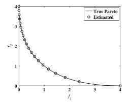
Fig. 4.8 A true Pareto front and the estimated front when setting  $f_1$  as the objective and  $f_2$  as the constraint.
