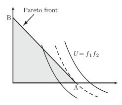
Fig. 4.10 Finding the Pareto solution with maximum utility in a maximization problem with two objectives
