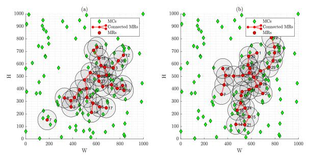
Fig. 6.6 Obtained topologies for transmission range 80m
