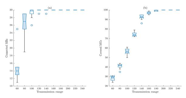
Fig. 6.10 Effect of the transmission range on coverage and connectivity
