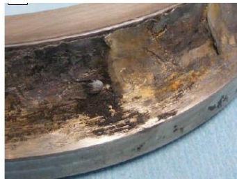
Figure 2. 10: Bearing surfaces damaged by adhesive wear (Vencl et al., 2017)
