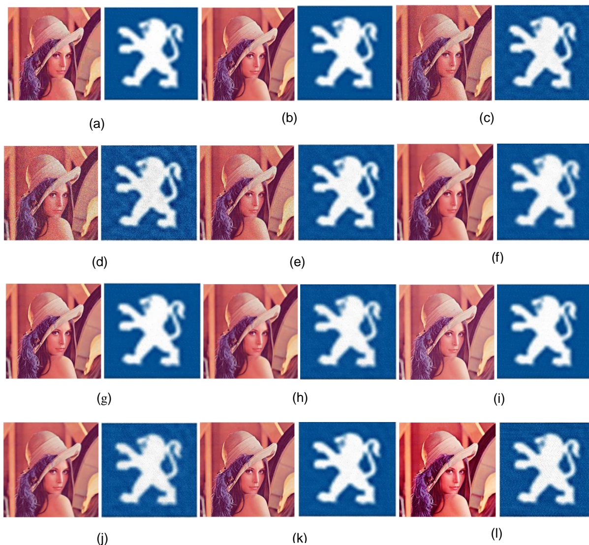
Figure 4.13 : L'image tatouée (Lena) et la marque extraite (Peugeot logo) après application d'attaques non géométriques : (a) JPEG(Q = 10), (b) JPEG2000 (CR= 5), (c) Salt and Pepper noise (0.05), (d) Gaussian noise (0.05), (e) Speckle noise (0.05), (f) Median filter (5×5), (g) Gaussian filter (5×5), (h) Mean filter (5×5), (i) Gamma correction (0.8), (j) Motion Blur (angle = 4, length = 7 ), (k) Sharpening (Radius = 2, Amount = 1), (l) Histogram Equalization (64 Bins ).
