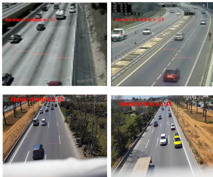
Fig. 11 Example of final vehicle detection counting system
