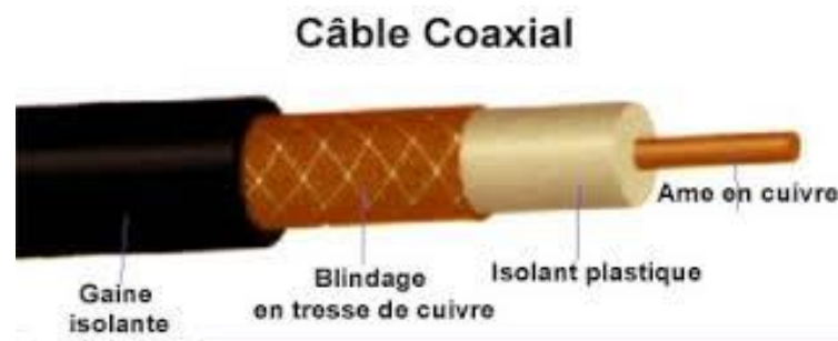
Figure 1-7 Le câble coaxial.
