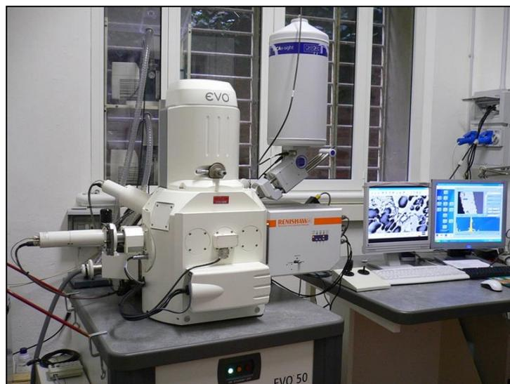
**Figure 3.7:** Microscope SEM (Zess Evo 50).
