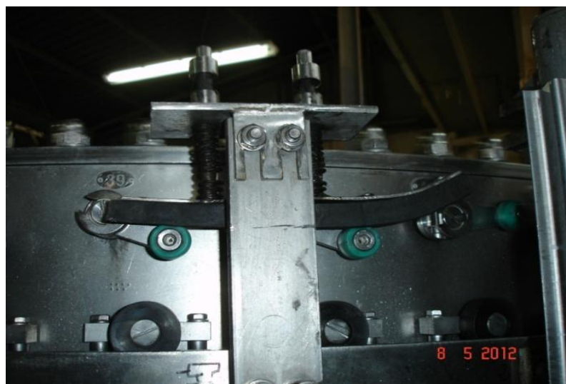
Figure 2.17. Came de fermeture des robinets.
