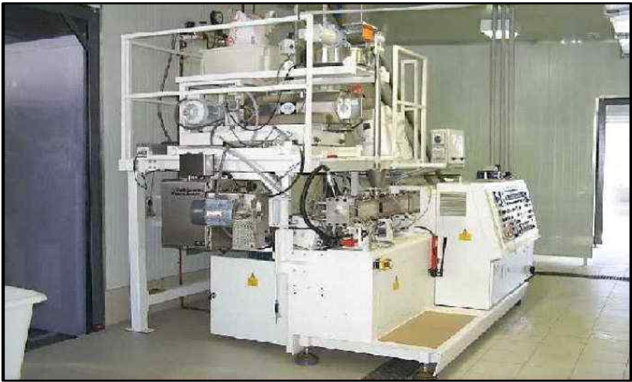
Fig. 10.13. Twin-screw food extruder
