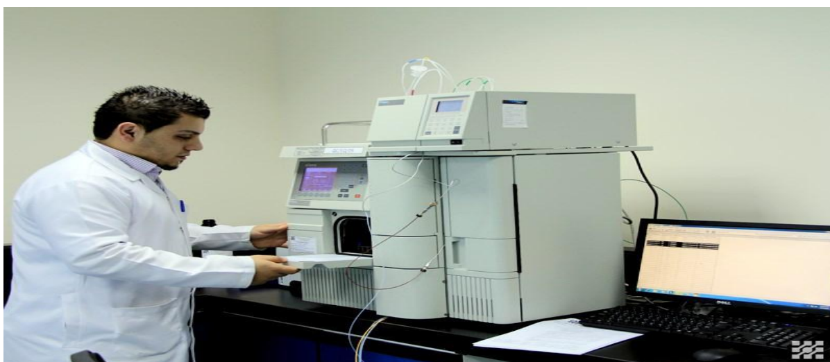
Figure 04: HPLC instrument used in the quality control of chemical drugs.
