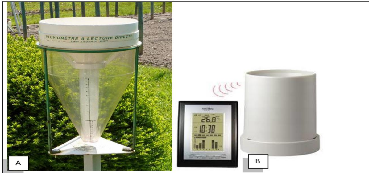
Figure 17. Direct-reading rain gauge (A). Electronic rain gauge (B).
