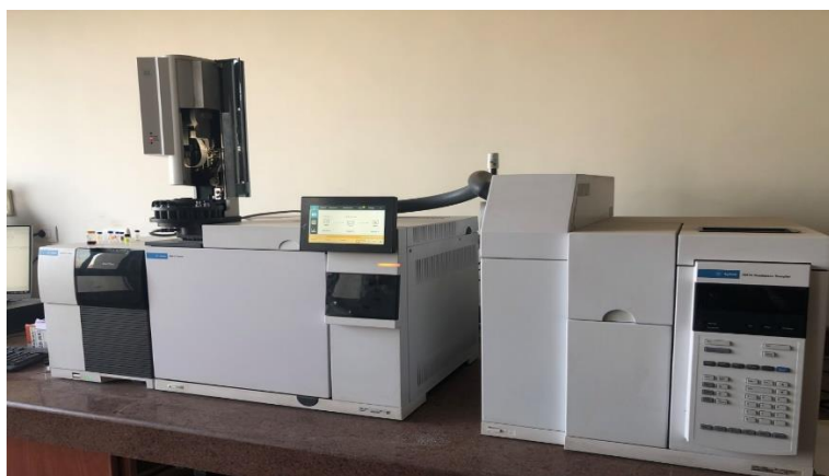
Figure A1.3. GC (Agilent 8890 System) coupled with MS (Agilent 5977B GC/MSD) NRC, Cairo, Egypt.
