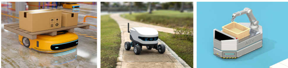
Figure 1.2: Different types of wheeled mobile robots (Differential drive in the left, Car-like drive in the center, Omnidirectional drive in the right).
