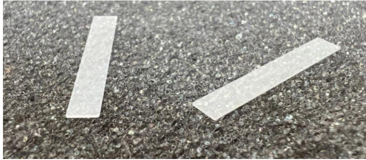
Figure III.2. BGO slices used for micromachining tests.
