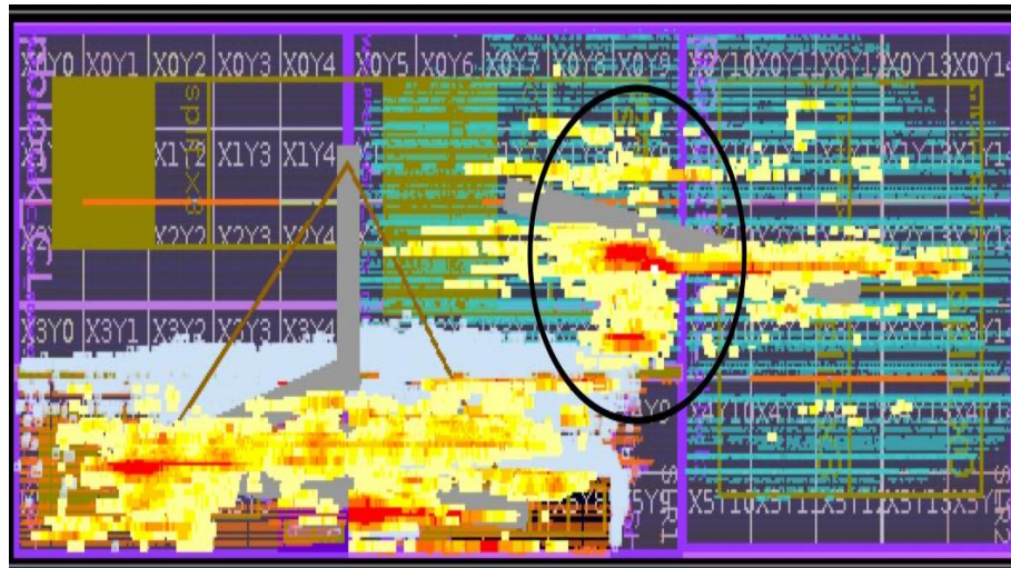
Fig. 3.20 Examples of routing congestion and optimization in FPGA Designs.
