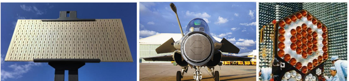
Figure 1.8. Examples of rectangular, circular, and hexagonal antenna arrays.
