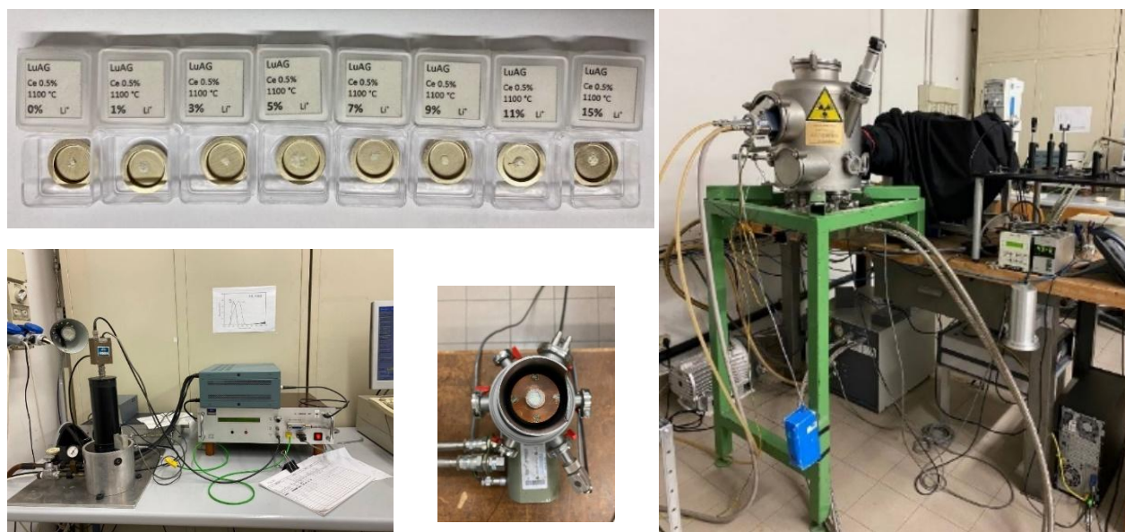
Figure II.9 wavelength-resolved thermally stimulated luminescence below and above room temperature, X-ray spectroscopy apparatuses – Unimib Italy .
