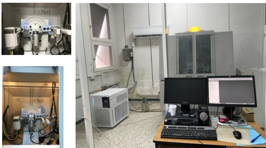
Figure II. 4 X-ray diffraction (XRD) technique a PANalytical X'Pert (Philips) PRO –CRNA Algiers.
