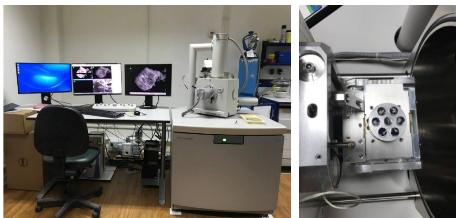
Figure II.5 JEOL JSM-5400 Thermoscientific Scanning Electron Microscope- ETAP Tunisia
