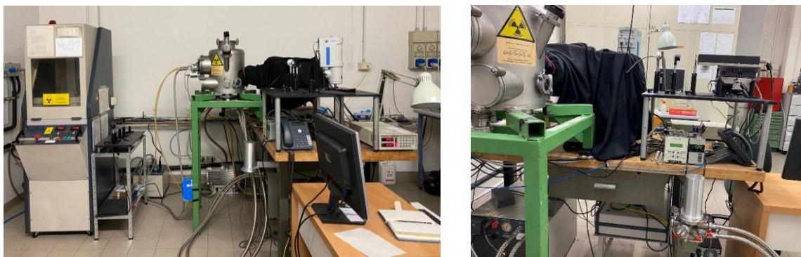
Figure II.7 Homemade instrumental setup for radio- thermo- and photo-luminescence- Unimib Italy .
