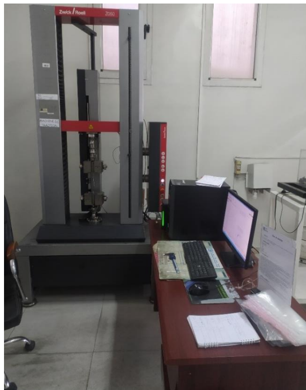
Figure 4.16: Machine de traction Zwick/Roell Z050.
