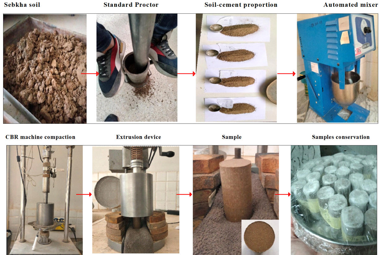
Fig 4-4. The Glimpses of Soil Sample Preparation.
