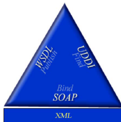
FIGURE 2.4 The relationship between XML/SOAP/WSDL/UDDI Cardoso et al. [2004]
