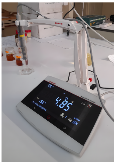
Figure III.17: Calibrated MODEL OHAUS equipment used for the electrical conductivity measurement
