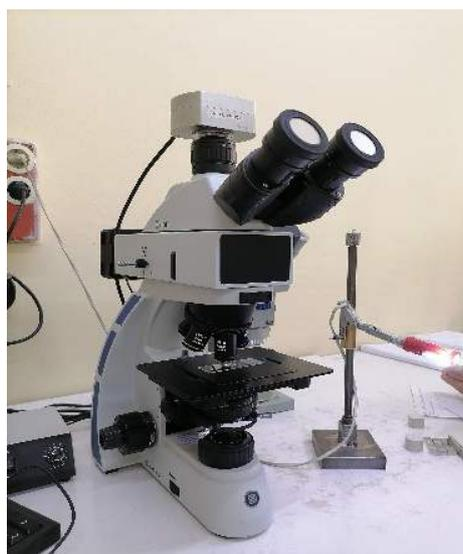
**Figure 3.6 :** Microscope universel Euromex de type OXION
