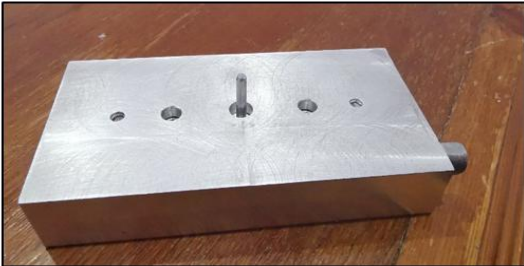
Figure IV.8 The Hollow Cylindrical Mold.
