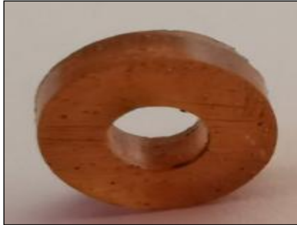
Figure IV.9 Sample Produced by the Hollow Cylindrical Mold.
