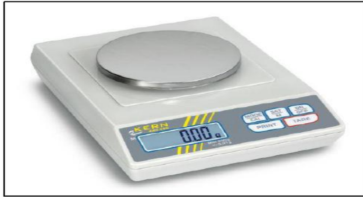
Figure IV.4 The electronic balance used for weighing the different proportions of powder
