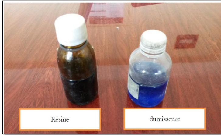
Figure IV. 22: The resin and the liquid hardener.
