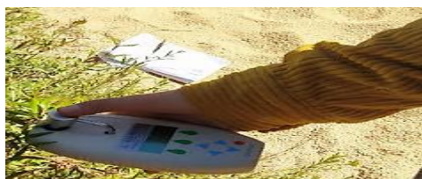
Figure 18: Measurement of leaf chlorophyll content using a portable CCM-200.
