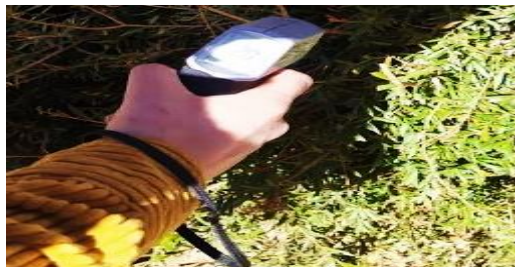
Figure16: Measurement of canopy temperature using infrared thermometer.
