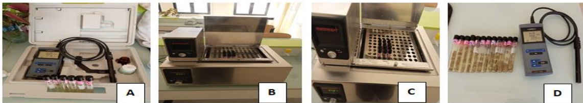
Figure 17: Determination of membrane stability index, A: record of electrical conductivity (EC1); B and C: place of the same samples in a water bath; D: record of the electrical conductivity (EC2).
