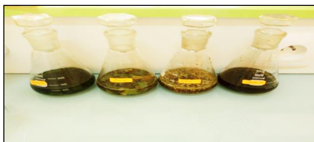
Figure 21: Maceration of two olive leaves in water and methanol.
