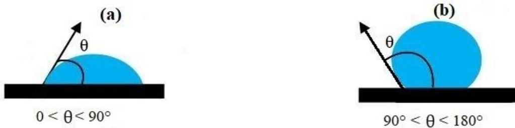
**Figure II.1 :** Angle de contact: surface hydrophile, (b) : surface hydrophobe
