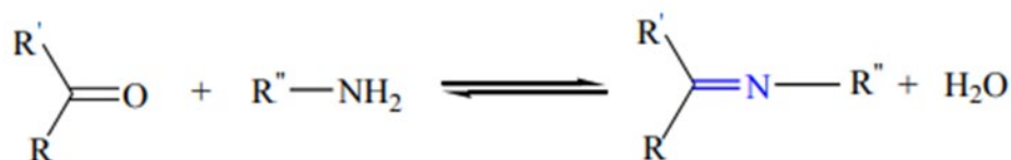
Scheme I.2. General reaction of Schiff base formation
