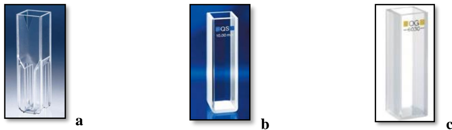
Figure. 10 : Different tanks. a: polystyrene tank, b: glass tank, c: quartz tank.
