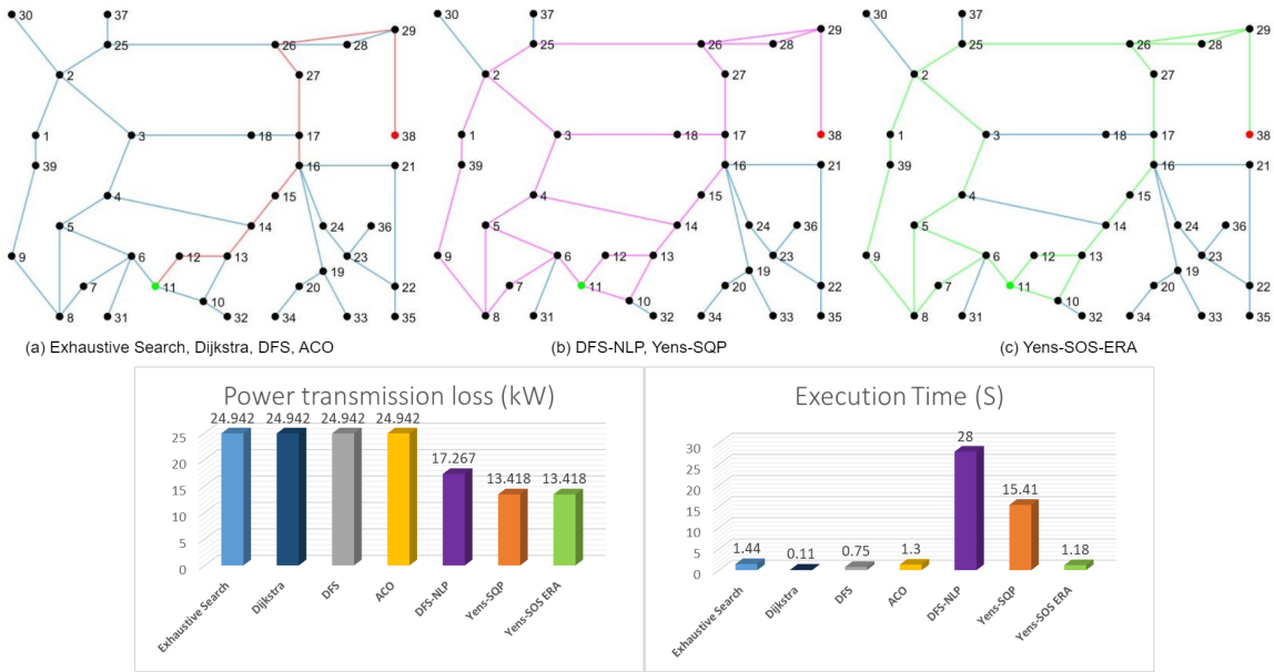
FIGURE 6.5: The selected least loss paths, power loss and execution time of each algorithm for the trading pair ( ER_{11}, ER_{38} ) in Figure 3.6.
