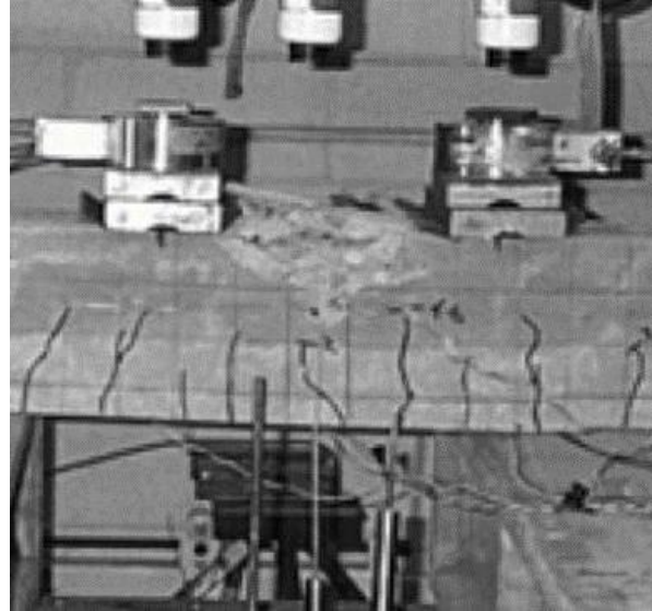
Figure. 1.10 Flexural Failure by Crushing of Compressive Concrete [83]
