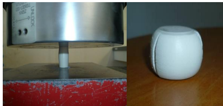
Figure 2.12 Failure mechanism in compressive adhesive testing. [113]
