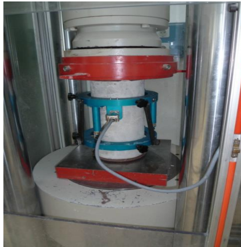
Figure 2.3 Measurement of the Young's modulus. [113]
