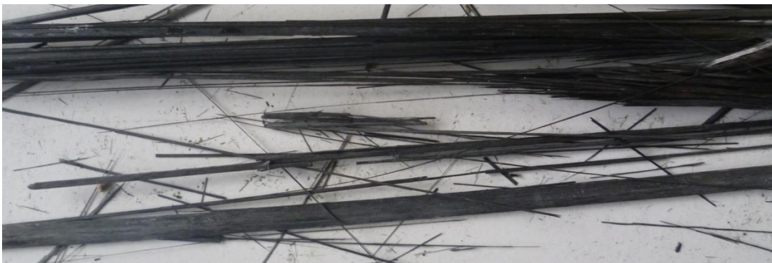
Figure 2.9 Failure mode of carbon reinforcements. [113]
