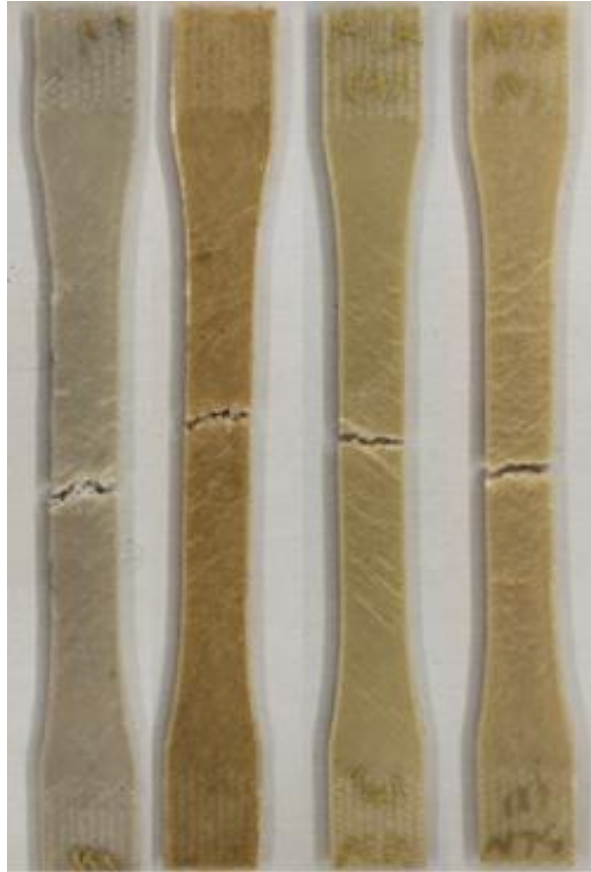
Fig. 5.7 Broken specimens after tensile test from left to right, PLA/PP, Un, Alk, and SLN respectively.
