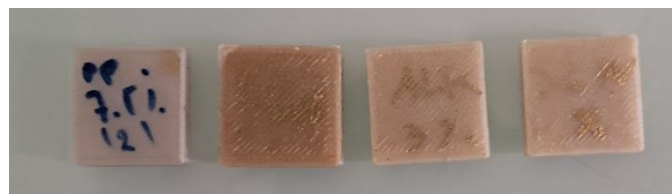
Fig. 3.8 Water absorption specimens.
