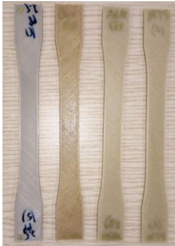
Fig. 3.6 Tensile test specimens: from left to right, PLA/PP, Un, Alk, and SLN respectively.
