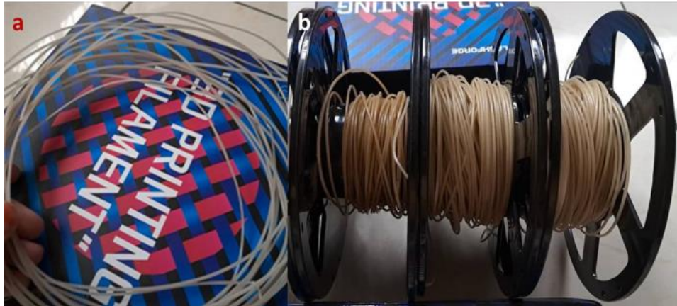
Fig. 3.5 The various composite filaments, (a) PLA/PP filament, (b) ArF reinforced filament, from left to right, Un, Alk, and SLN respectively.
