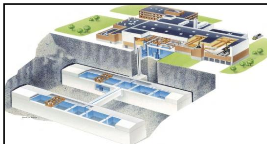
Fig. 1.8. The CLAB facility in Sweden for underground storage (about 30m deep of spent fuel under water).
