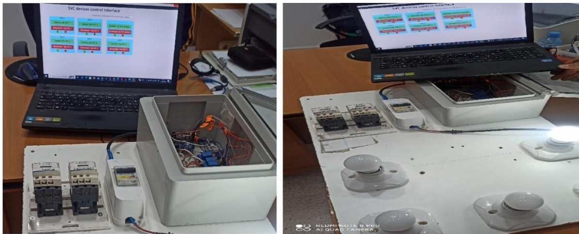
Figure 6.13. Practical implementation for controlling SVC devices
