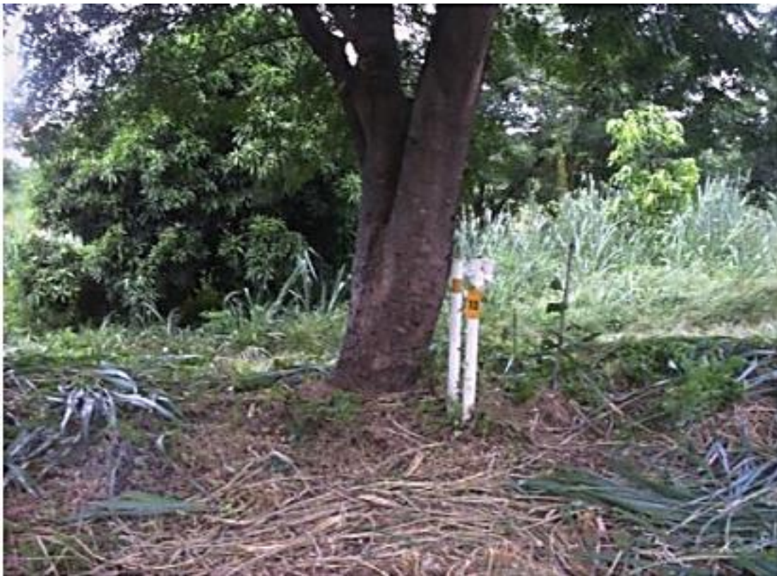
Figure II. 4. Station of environmental TLDs used in Instituto de Engenharia Nuclear-IEN for environmental kerma assessment [56].
