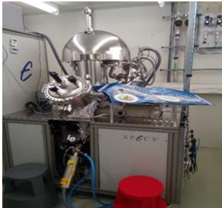
Figure IV.16: Ultra-high vacuum system with an attached XPS system.
