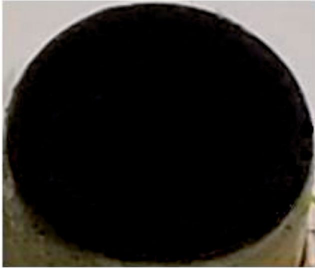
Figure 10. Image of PAni/CdTe composite film on XC70 mild steel after 6 months of electrodeposition.
