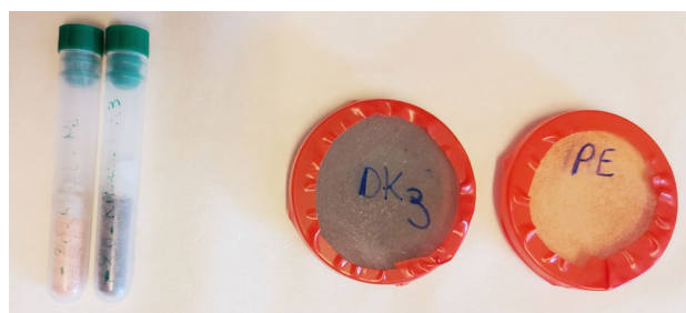
Fig. 3 Tubes and petri dishes used for gamma measurements
