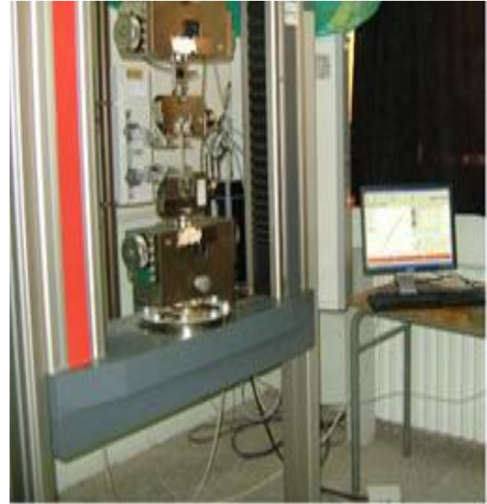
Figure 3.11: Machine de traction Zwick Rowell 100 KN.
