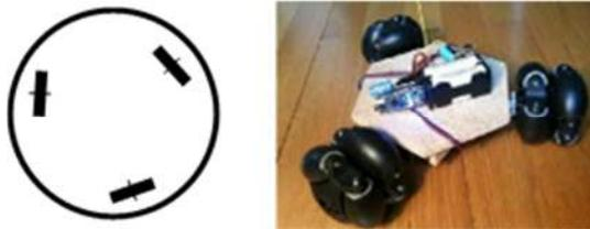
**Figure I.4** Robot mobile de type omnidirectionnel.
