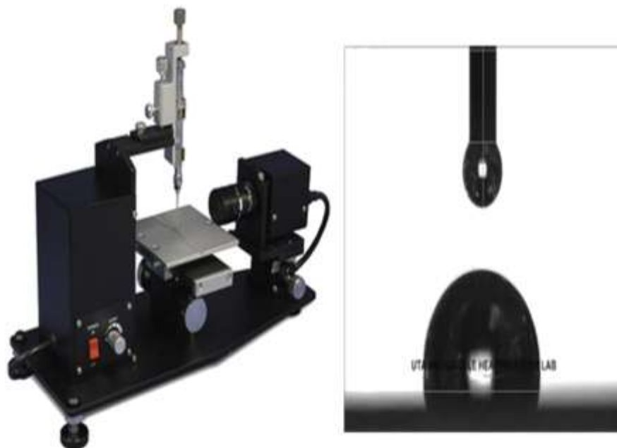
Figure 2.27 Measurement technique of Digi Drop[235].
