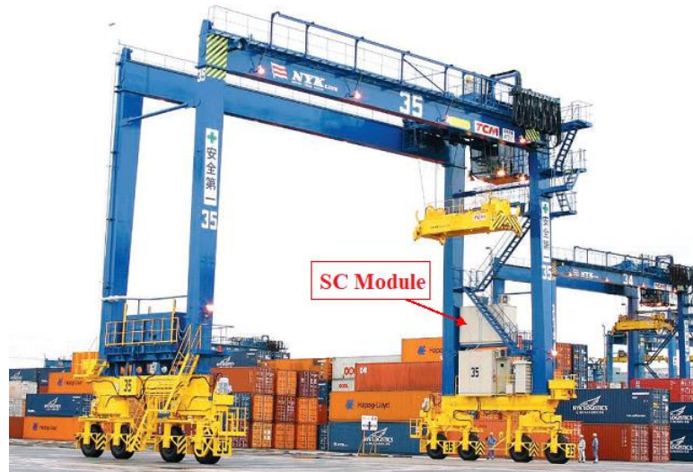
Figure 3: Airport crane in Japan combining a diesel engine and supercapacitor modules. [22]
