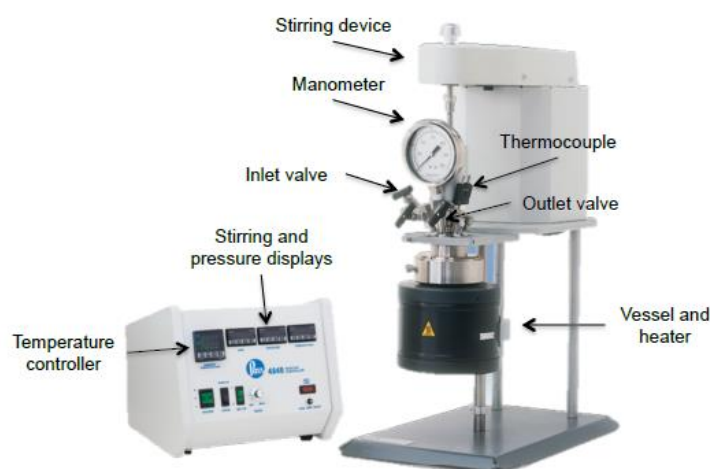
Figure II.4. Parr reactors used for the hydrogenation reaction
