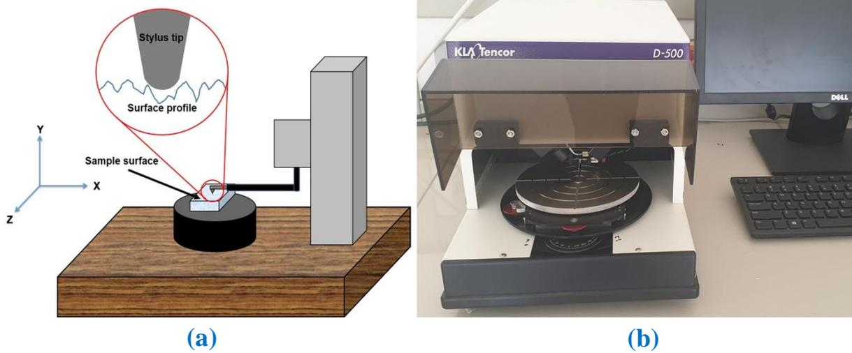
**Figure II.10:** The principle of sensor contact profilometer (a) and the used AlphaStep D-500 Stylus Profiler (b).
