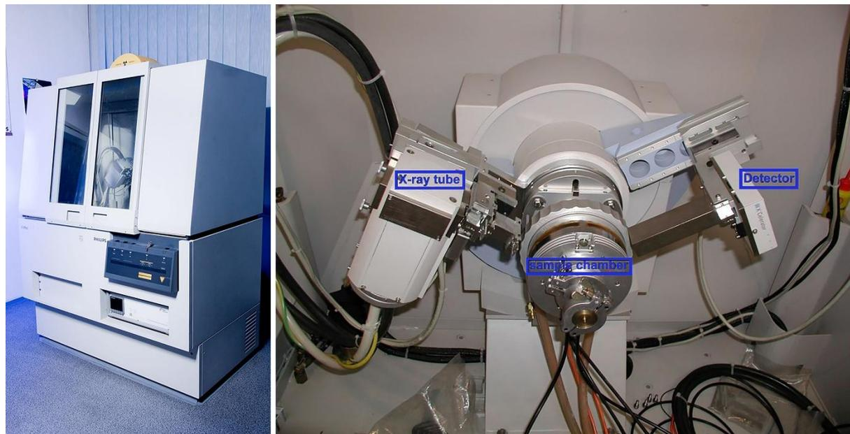
**Figure II.8:** The used Philips X'Pert X-ray diffractometer.
