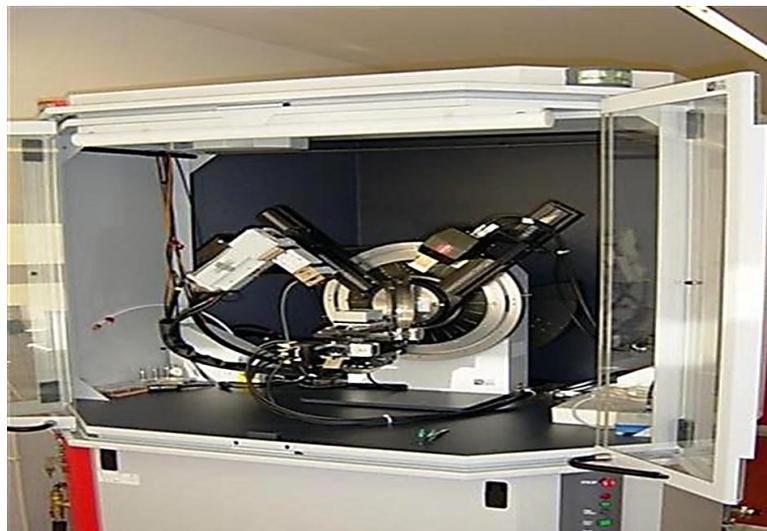
**Figure III. 17 :** Diffraction des rayons X (DRX) - Bruker D8 Discover.
