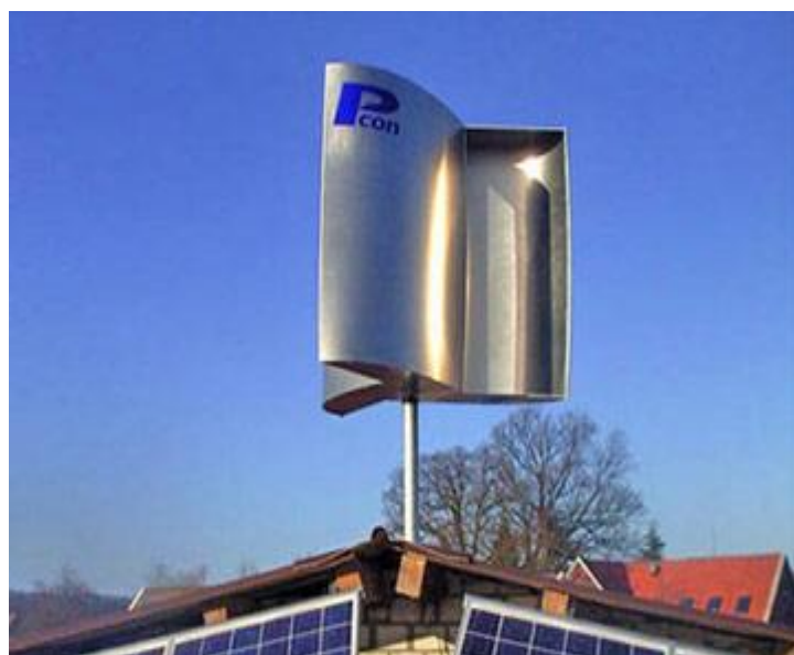
Figure 5.3 Savonius type vertical axis wind turbine
