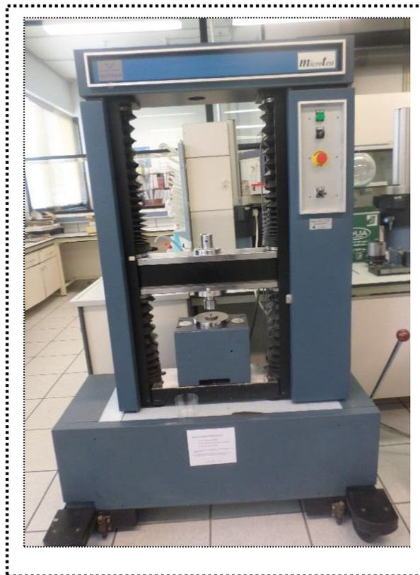
**Figure IV.18 :** Machine de traction Microtest
