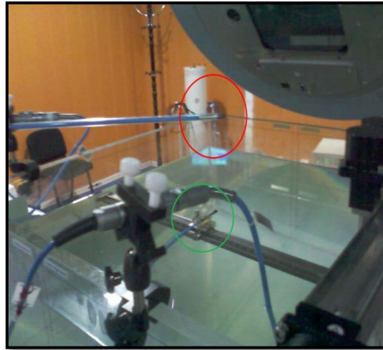
Figure IV.11: Relative chamber fixed on the movable arms (green circle at the bottom) and reference chamber positioned on the edge of the selected field (red circle at the top)
