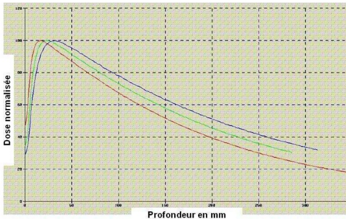
Figure.II.8: Percentage depth dose (PDD) 6, 10 and 18 MV beams (Precise, Elekta®). The maximum depth is 17 mm, 24 mm and 32 mm respectively, for the energies mentioned above.
