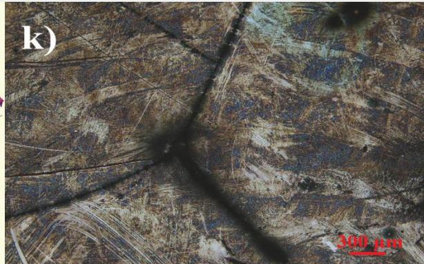
**LEMG124**  $R_a = 18,67 \mu\text{m}$ ,  $R_q = 24,58 \mu\text{m}$ ,  $R_z = 137,51 \mu\text{m}$ .
