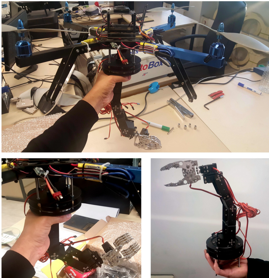
Figure B.1: Initial developed platform of the Quadrotor manipulator: The Quadrotor is equipped with a 7 degree of freedom robotic arm.
